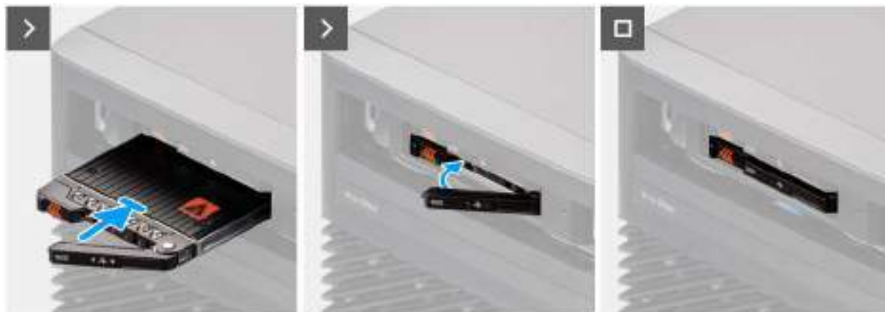
Figure 50. Installation du support de disque SSD M.2
