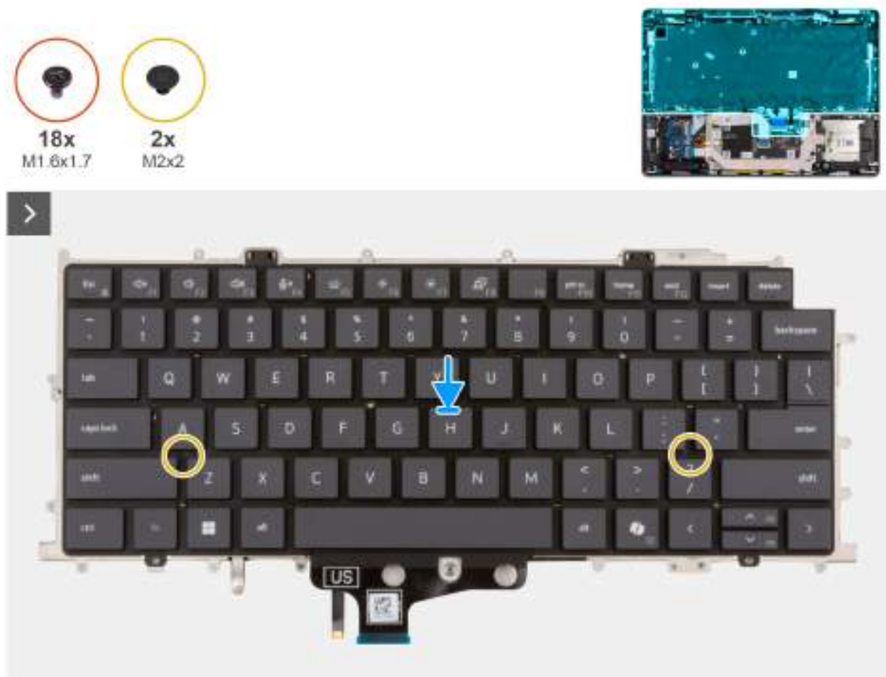
Figure 100. Installation du clavier
