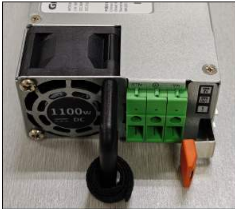
Figure 21. Connector on the ThinkSystem 1100W -48V DC Hot-Swap Gen2 Power Supply v2 (4P57A89415)
