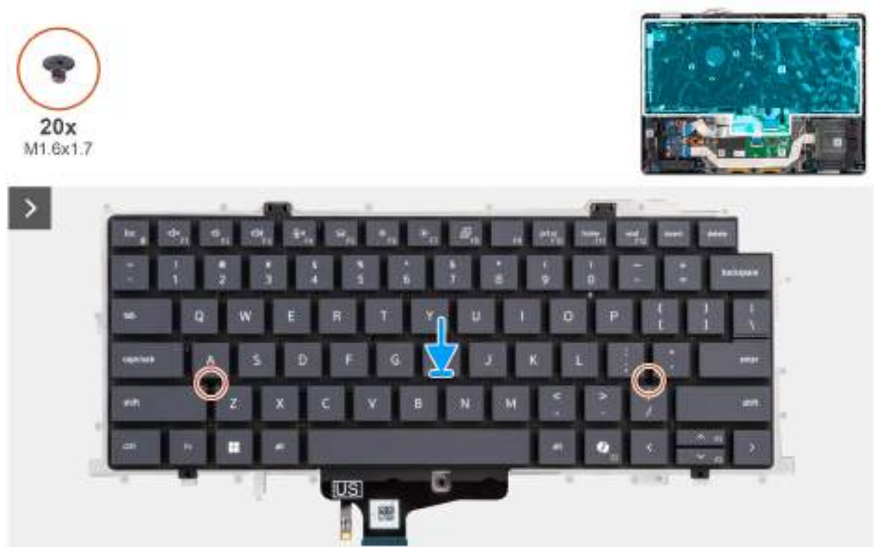
Figure 99. Installation du clavier
